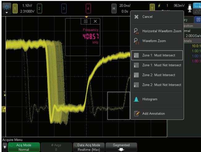
Figure 11. Draw a zone (box) around the anomaly.
