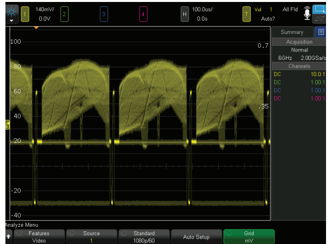
Figure 45. Triggering on a 1080p/60 signal.
