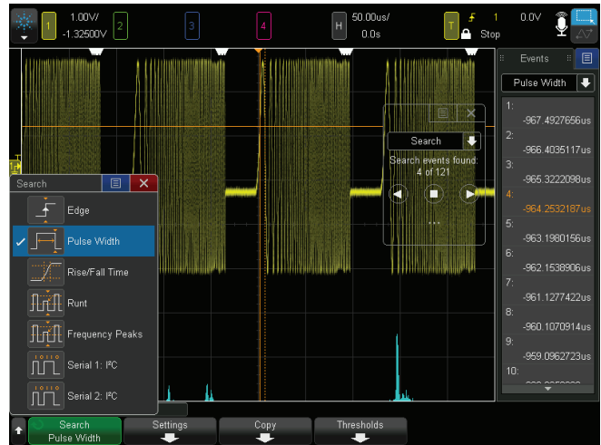
Figure 42. Searching for and navigating to a specific pulse width.
