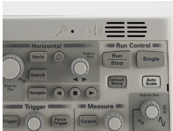
Figure 39. Voice control microphone and speaker.
