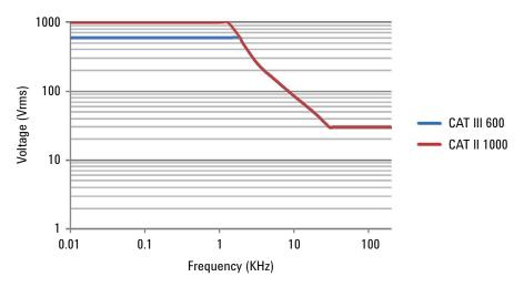
Figure 5. Maximum safety voltage for scope reference to earth
